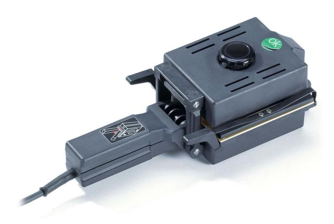
The PT-100 is a hot-pressing device for Thermofix joining of Habasit belts and tapes up to a width of 100 mm and a thickness of 6 mm. The lower press plate is heated and is equipped with a detachable set-up plate with clamping springs for secure positioning of the belt ends. Its knuckle joint mechanism allows easy adjustment for different belt thicknesses. Together with the integrated pressure equalization pad, it ensures reliable hot pressing for even the most demanding glued belt joints.
