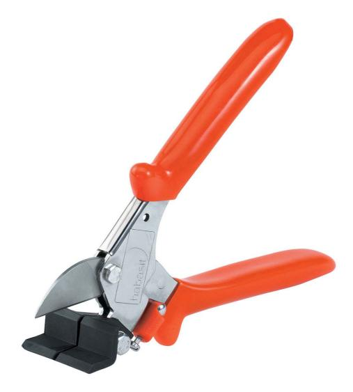
The cutting device S-16 is a manual cutting tool to cut Polycord round belts to the required length before the Quickmelt joining procedure takes place. The S-16 allows to perform a proper right-angled cut up to 15 mm/0.6 *in.* diameter.
